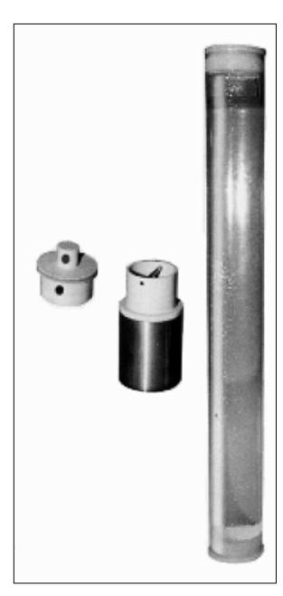
This device allows quick and easy sampling of water in piezometric wells, while at the same time preserving the surface structure and any supernatants. The gauge body acts as both sampling device and receptacle for the storage and transport of the sample, thus preserving the latter's integrity. Once the sample has been taken, the upper and lower ends of the device are closed simply using the two plugs supplied.
